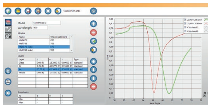
Figure 5. MP-SPR Navi™ LayerSolver™ can be used to fit measured SPR curves to determine thickness and RI of the deposited layer.
