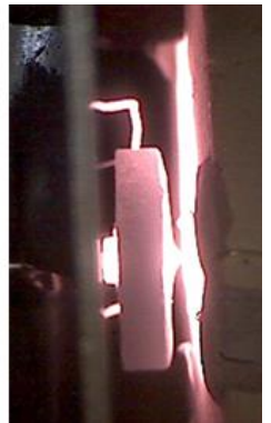
The horizontal high temperature configuration of the NanoTest (left) and a close-up view of an indenter and sample at 950 °C in vacuum (right). (Figures above left and below left courtesy of Dr Jeff Wheeler, ETH Zurich.)
